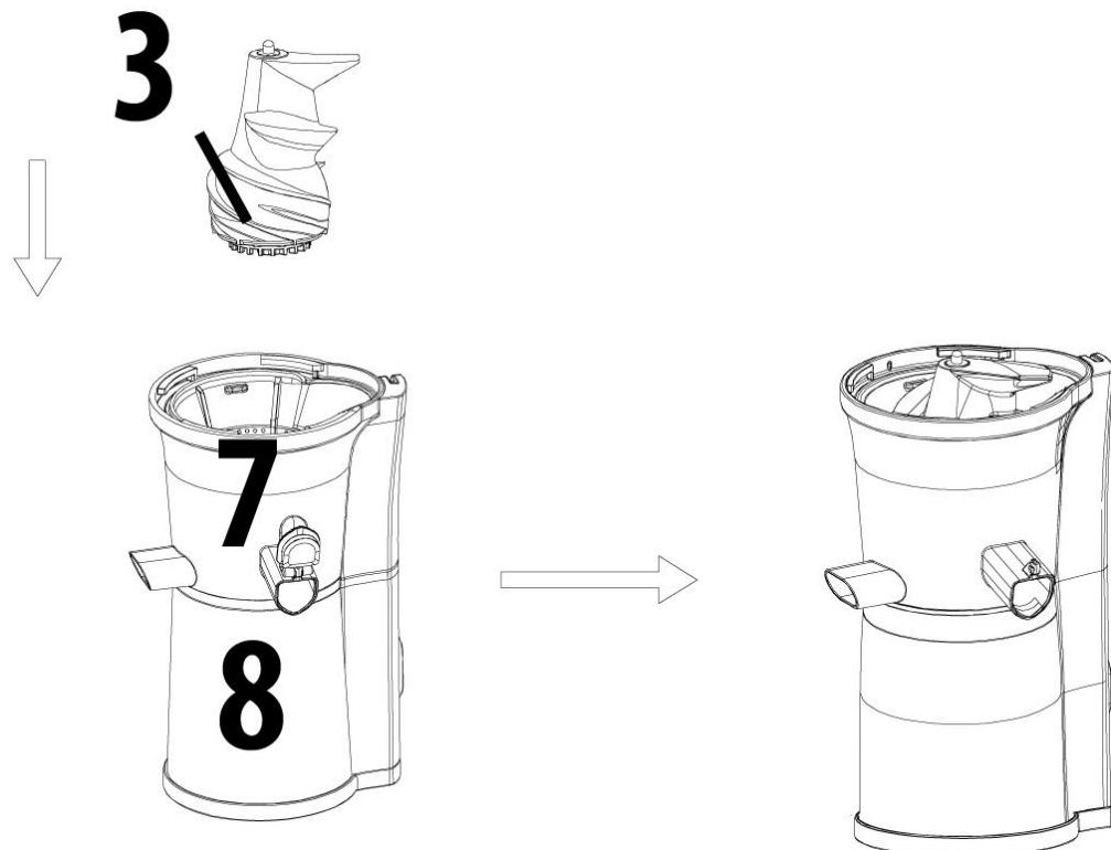
Then place the pressure auger (3) into the already assembled juicing strainer / sorbet strainer, press it down and rotate until it latches.
