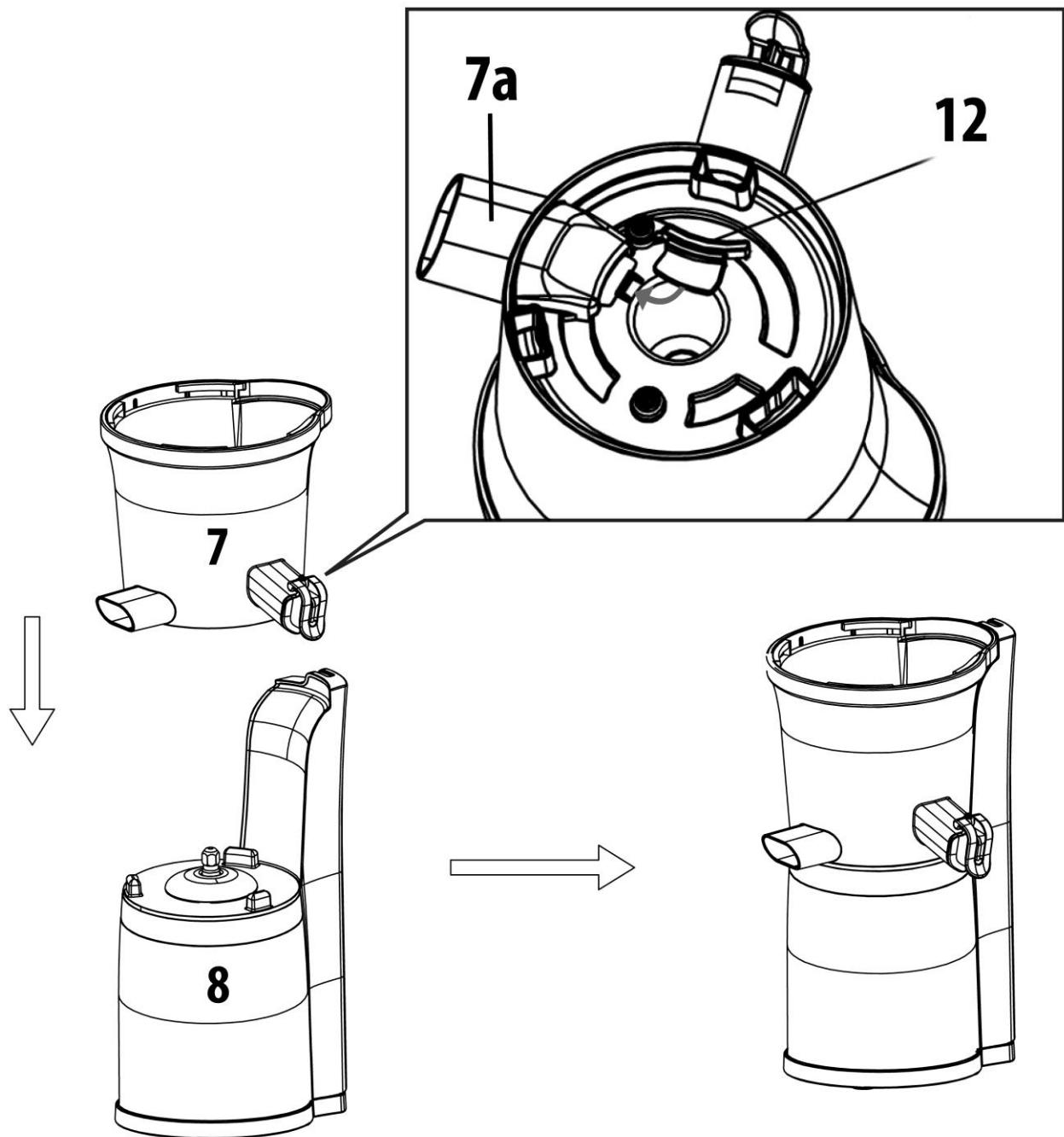
Check that the silicone plug (12) is placed in the outlet for residues (7a), which is on the underside of the middle part with outlets (7). Place middle part with outlets (7) on motor unit (8).
