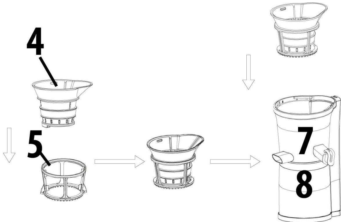
**For making of juice:** Place the juicing strainer (4) into the wiper basket (5) and rotate it lightly until the wiper basket latches. Then place the juicing strainer with wiper basket into the middle part (7).
